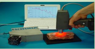
Figure 2 is an example of an actual laser product being used to measure the quality of a meat product.
